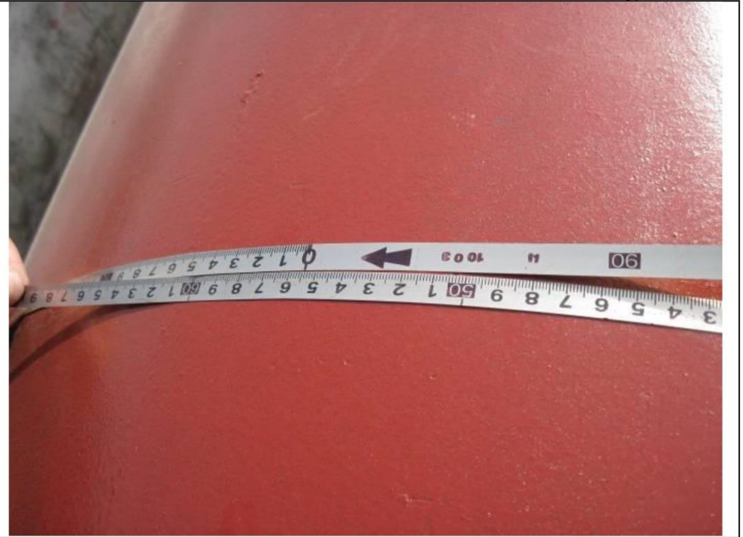
Measuring OD of pipe body
