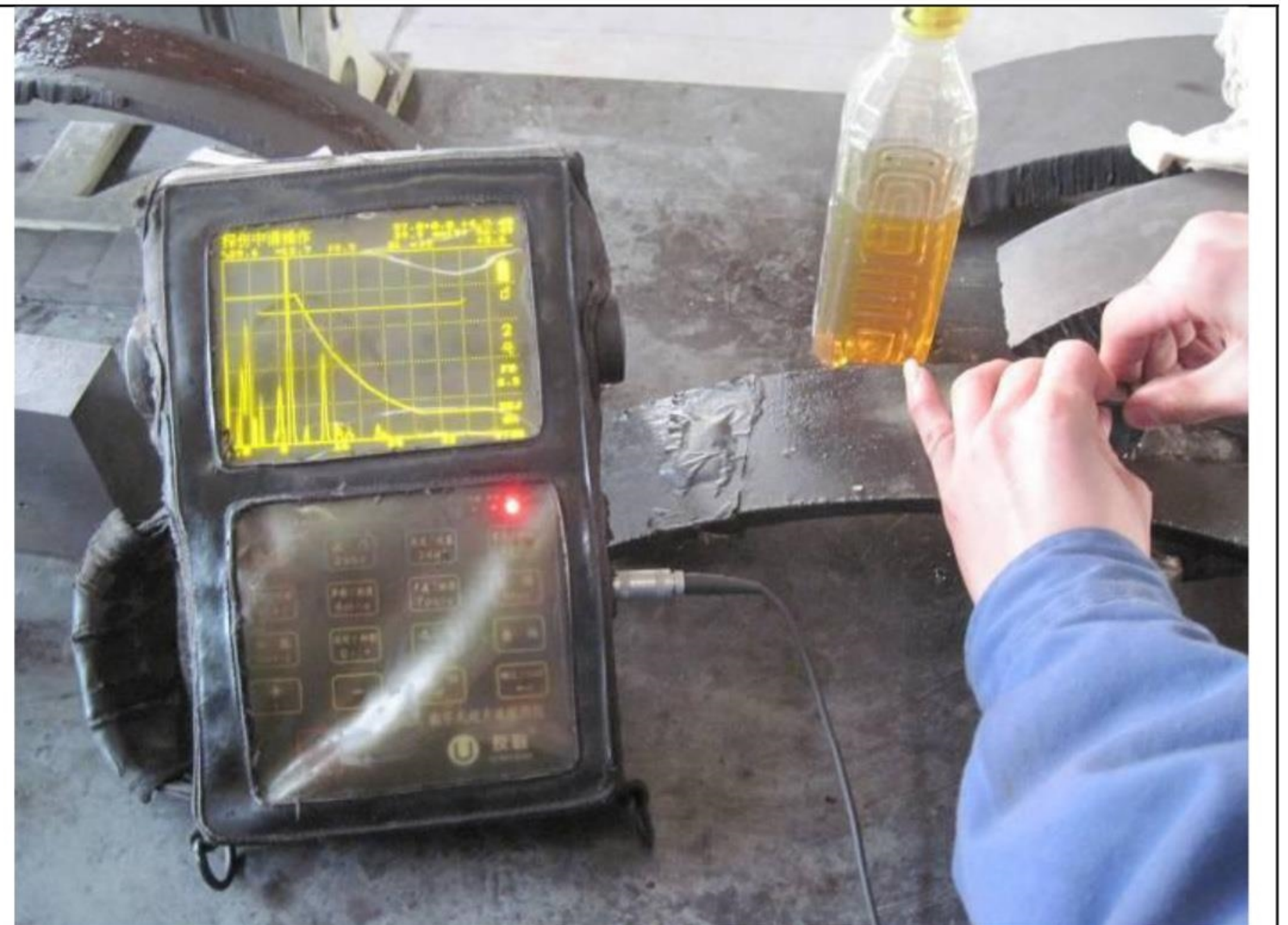
Ultrasonic fault detector calibration
